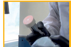
Clean Teflon piston and metal cylinder.
